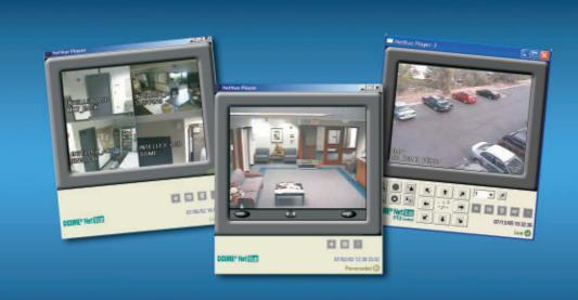
C•CURE NetVue is an option within C•CURE 800/8000 that provides seamless integration with a variety of digital video management systems (DVMS). This integration not only allows users to tie an event generated on C•CURE 800/8000 to a video clip, but also to automatically activate events based on alarms received from the DVMS.
